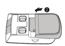
**Step 1:** Plug the battery connector securely into the socket inside the battery compartment. Insert the battery with the label **THIS SIDE UP** facing up onto the battery compartment.
